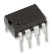
Your IC should have a notch on one end. Install the IC so the notch matches the one printed on the board. If the supplied IC does not have a notch, it will have a small dot on one corner. Install the IC so that dot is on the same end as the notch printed on the board
