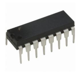
Your IC should have a notch on one end. Install the IC so the notch matches the one printed on the board. If the supplied IC does not have a notch, it will have a small dot on one corner. Install the IC so that dot is on the same end as the notch printed on the board
